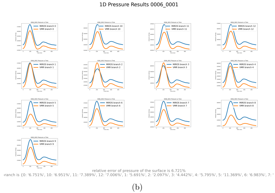
Figure 4.10: 1D flow and pressure plots at all outlets for model 0006.0001, index 1 in Tables 4.3, 4.4, for which errors where the highest. Comparing the machine learning based constructed model with a manually constructed one (ground truth).
